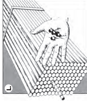
Uranium is formed into ceramic fuel pellets about the size of a fingertip.
