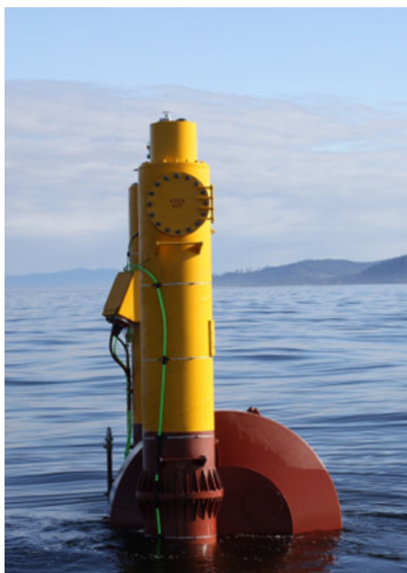
Northwest Energy Innovations verified the ocean wavelength functionality of the Azura device (previously called WET-NZ) through wave tank testing and a controlled open-sea deployment of its 1:2 scale device.
