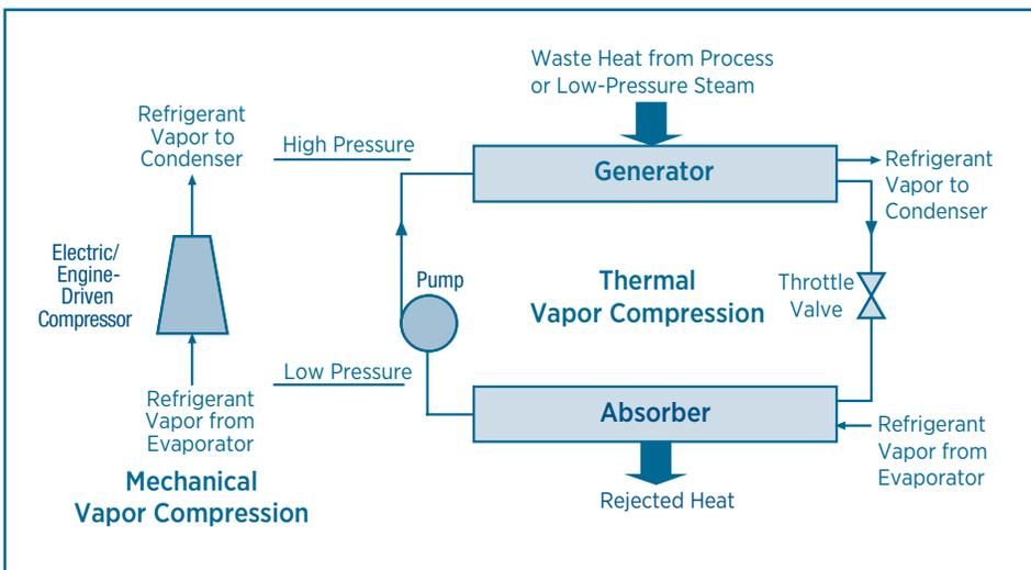
\*The evaporator and the condenser, required for both systems, are not shown in the figure.
