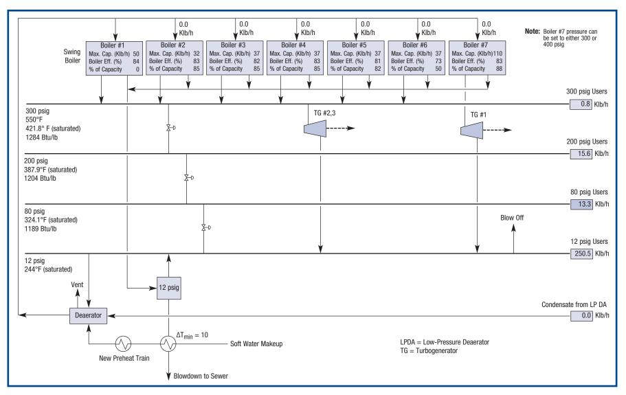
Figure 2. Simplified Schematic Flowsheet of Combined Heat and Power System for a Sugar Refinery
