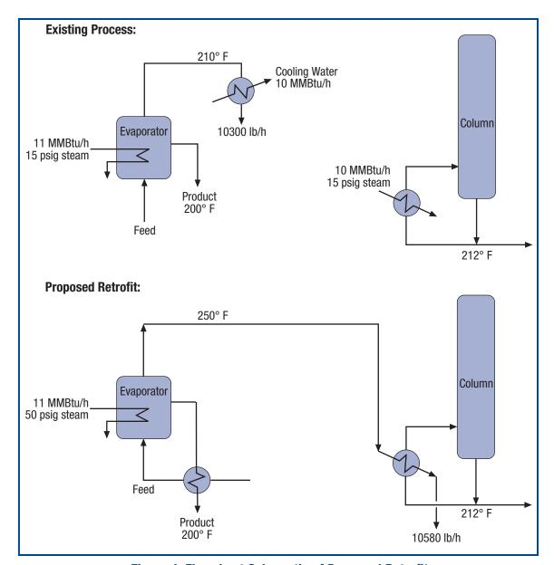
**Figure 4. Flowsheet Schematic of Proposed Retrofit**
