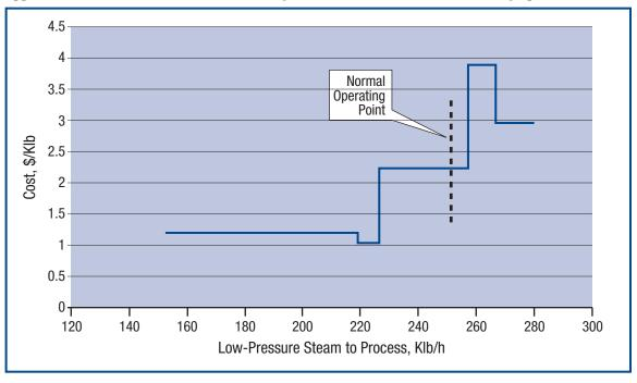
Figure 3. Variation of Net Low-Pressure Steam Cost (Marginal) with Consumption Rate
