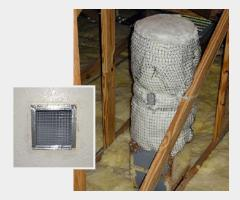
Each lab was configured with four controllable ceiling leakage sites providing ~70% of leakage area.
