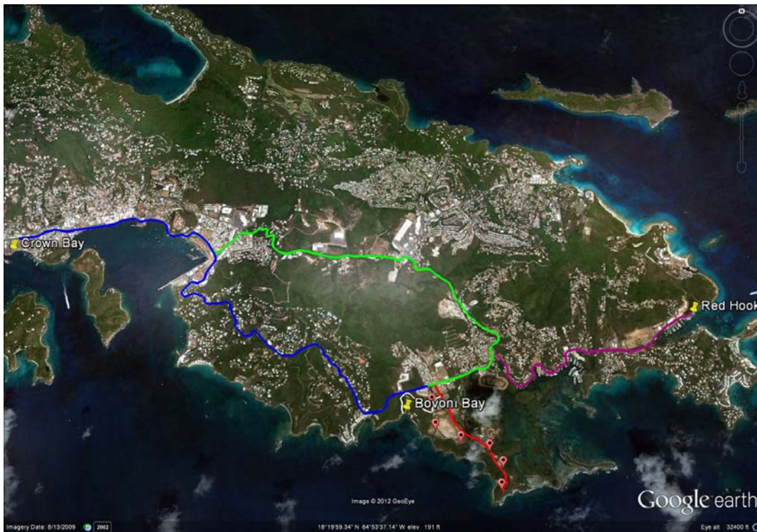
Figure 23. Possible equipment drop points and overland transport routes, including likely problem turns
