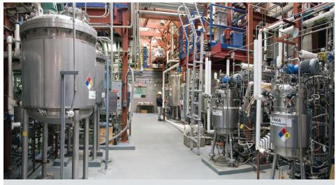
Researchers at NREL's Integrated Biorefinery Research Facility study biochemical processes for the conversion of lignocellulosic biomass. NREL can process biomass at a scale of 1 ton per day. *Photo: NREL/16330*
