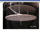
Antenna (4" monopole) mounted to baffle plate on tank lid
