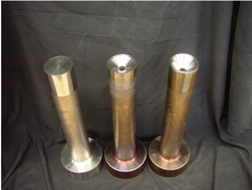
Extrusion stems for indirect extrusion, showing (left to right) spare blank, 30° and 45° dies
