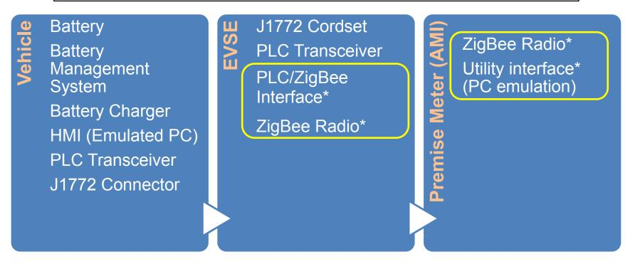
**Test Scenario**: Send message from vehicle and receive at utility interface
