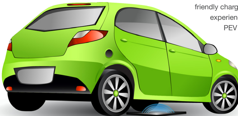
PEV wireless charging over transmitting plate. (Courtesy of Oak Ridge National Laboratory.)
