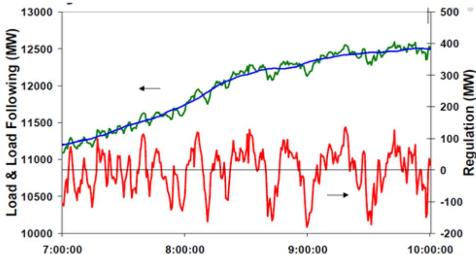
**Figure 1-3. Regulation and load following during normal conditions.**
