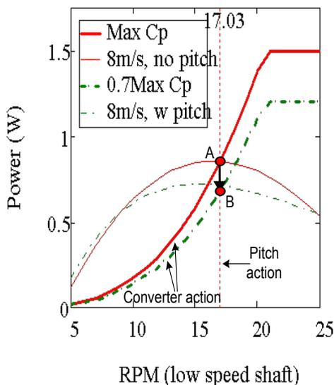
**Figure 3-23. Operating points for the proposed control.**
