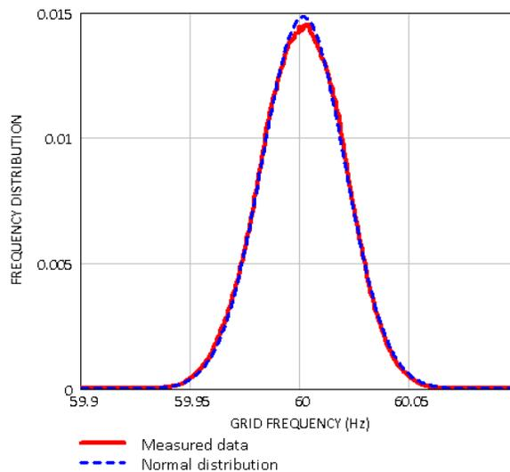
**Figure 3-38. Distribution fitting for continuous frequency data.**
