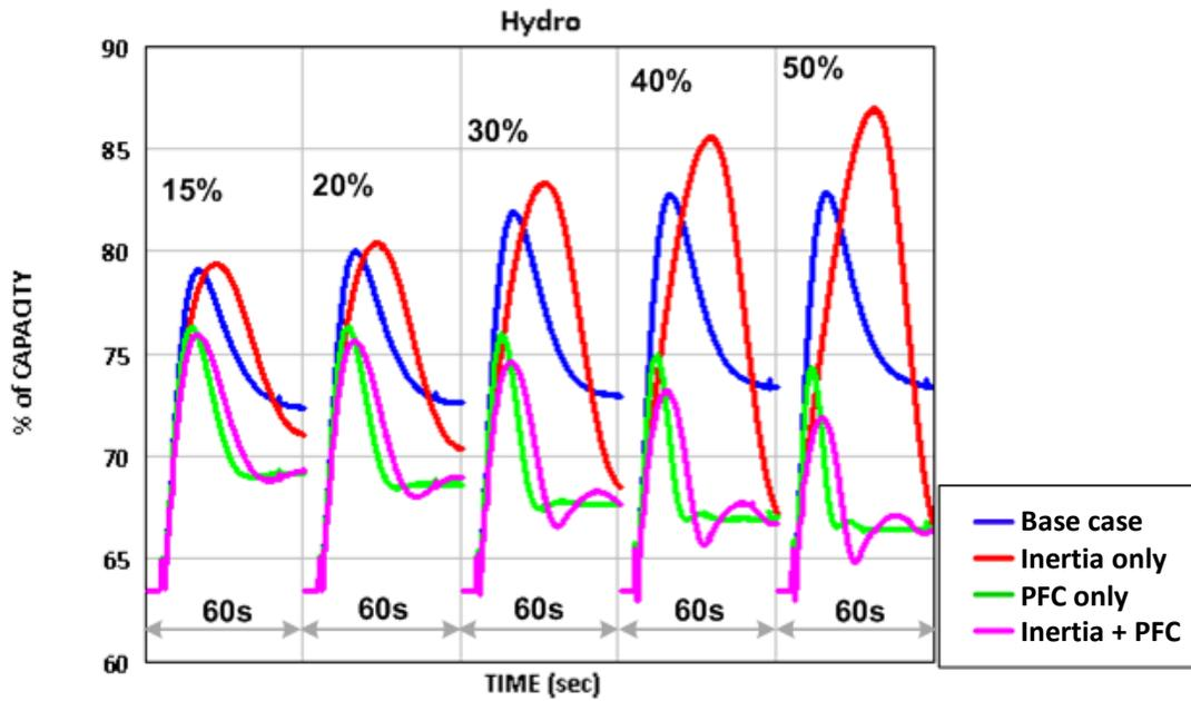
Figure 3-51. Frequency response contribution from hydro unit.
