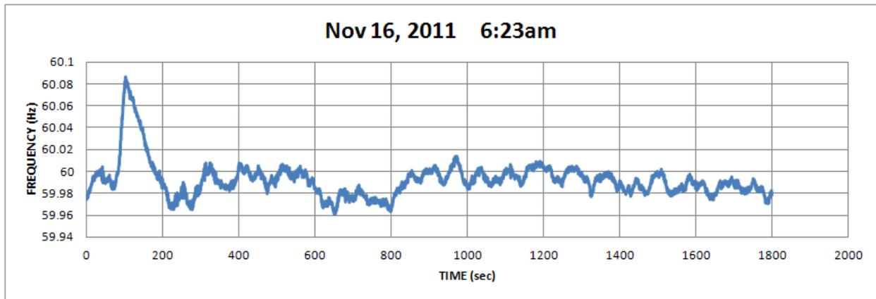
**Figure 3-34. Example of WECC over-frequency event.**
