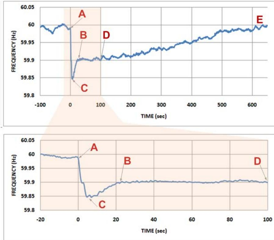
Figure 3-31. Typical WECC frequency response (August 6, 2011 at 11:19 am).
