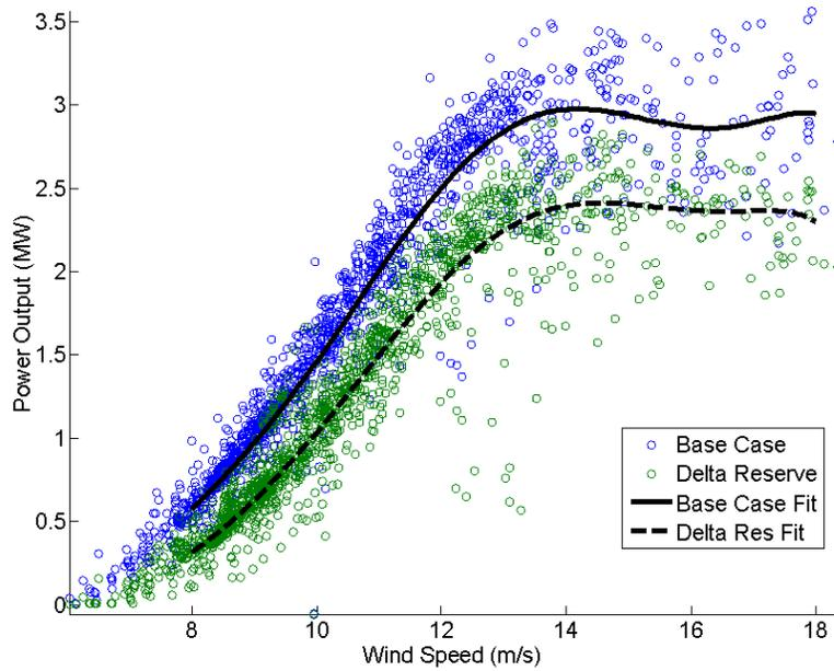
Figure 3-17. Output power comparison between the base case and delta reserve power of a Type 2 wind turbine based on the dynamic simulation with  $\Delta P_{reserve} = 20\%$  of the rated power.
