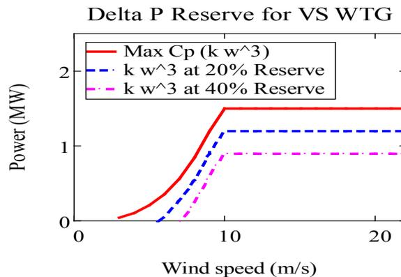
**Figure 3-22. The reserve power for a variable-speed WTG using two different methods.**
