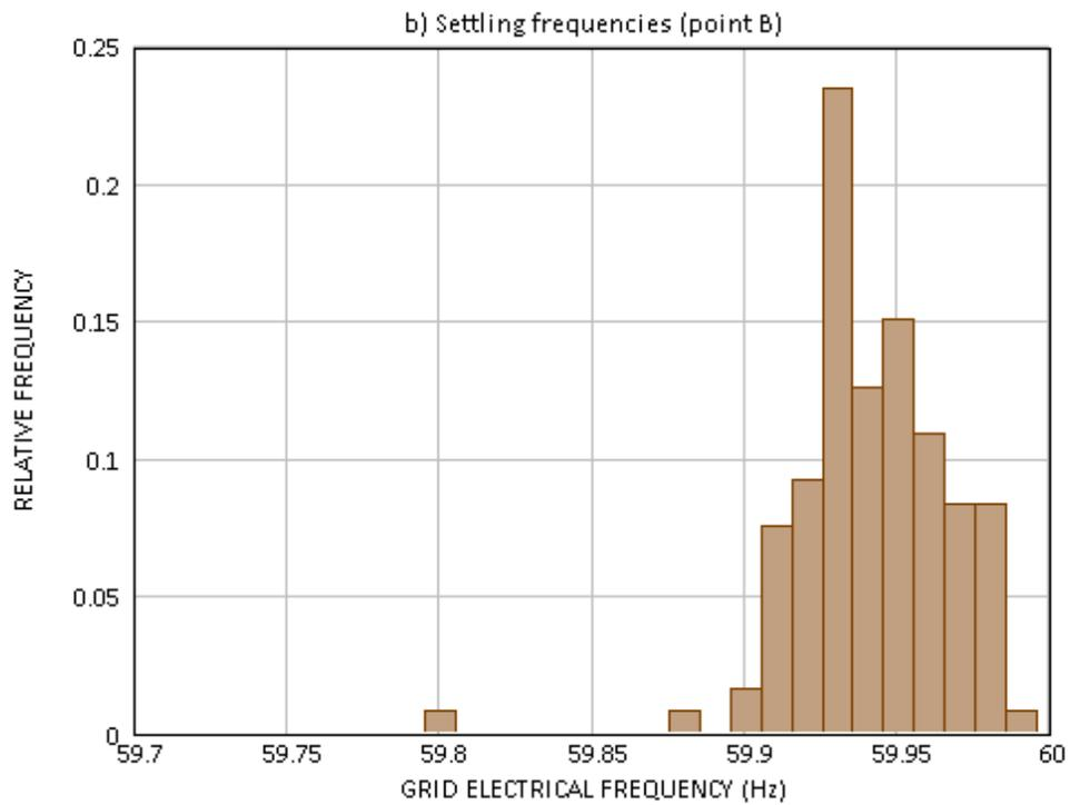
**Figure ES-4. Distribution of low-frequency event data. Point C is the frequency nadir and point B is the settling frequency.**
