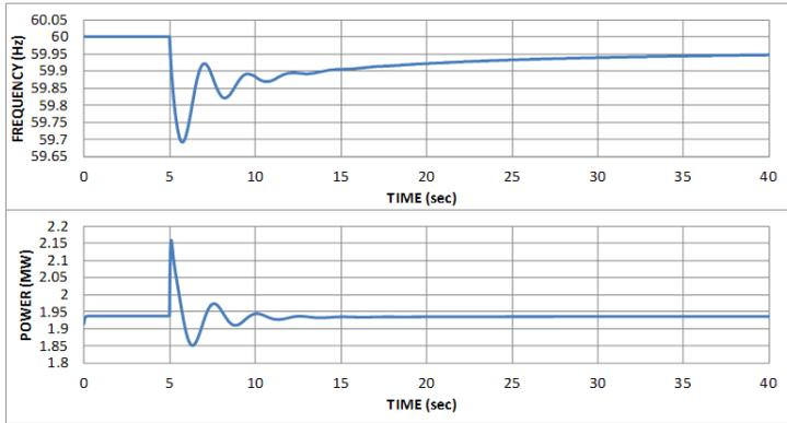
**Figure 3-8. Frequency response for Type 1 WTG connected to a power system with low inertia.**
