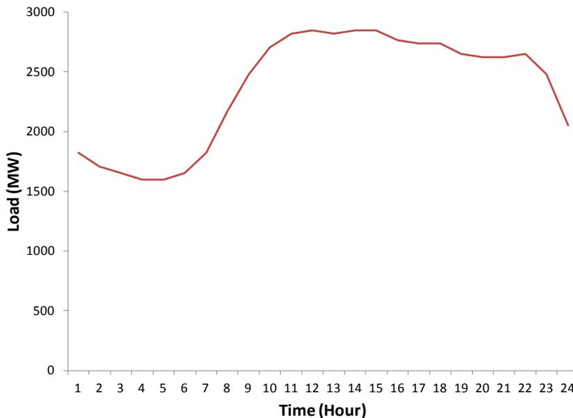
Figure 2-4. Load profile from peak load day.
