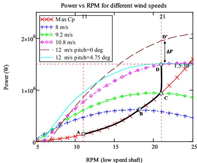
**Figure 3-19. Illustration of kinetic energy transfer during a frequency decline for Type 3 and 4 WTGs.**
