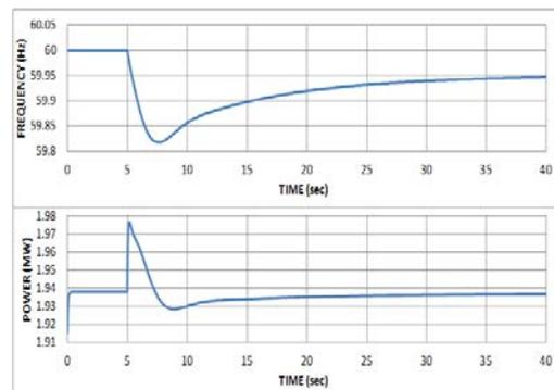
**Figure 3-6. Frequency response of Type 1 WTG connected to a power system with large inertia.**
