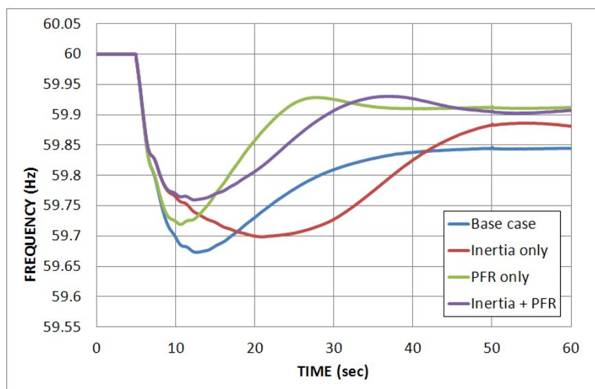
Figure 3-43. WI frequency response for 20% wind power penetration.
