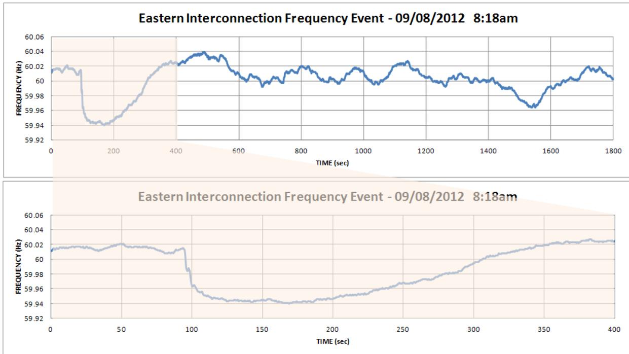
**Figure 3-35. Example of EI under-frequency event.**
