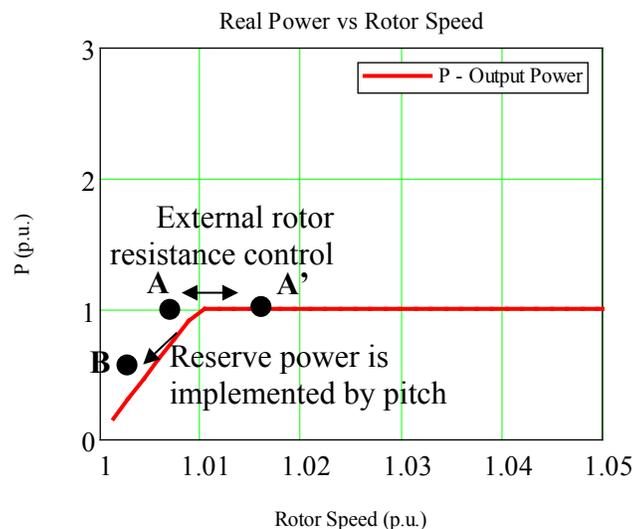
Figure 3-12. Output power versus rotor speed (Type 2 WTG).
