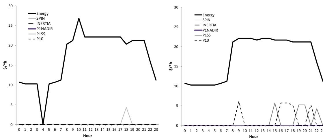
**Figure 2-5. Prices for BC1 (left) and BC2 (right). Prices are in (\$/MVAs-h) for inertia and (\$/MWh) for all other services.**
