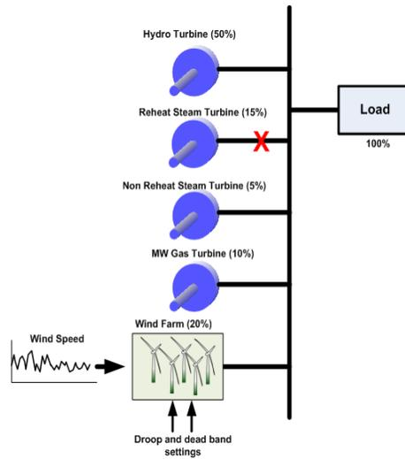
**Figure 3-4. Simplified governor-based power system model.**
