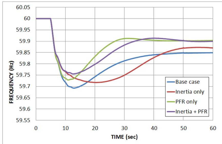
Figure 3-42. WI frequency response for 15% wind power penetration.
