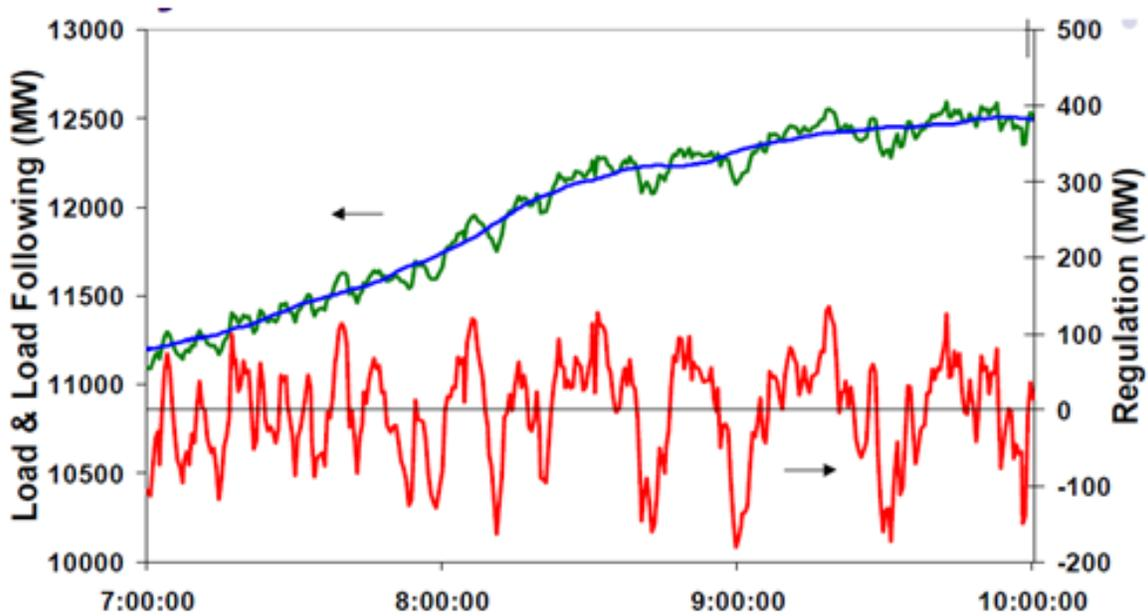
**Figure ES-3. Regulation and load following during normal conditions.**
