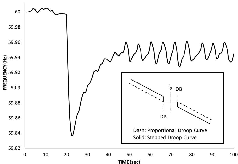
**Figure 2-3. Simulated frequency response following disturbance with units having a stepped droop curve governor response and illustration of proportional vs. stepped droop curves.**
