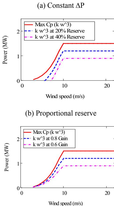
**Figure 3-14. The reserve power held using two different methods.**
