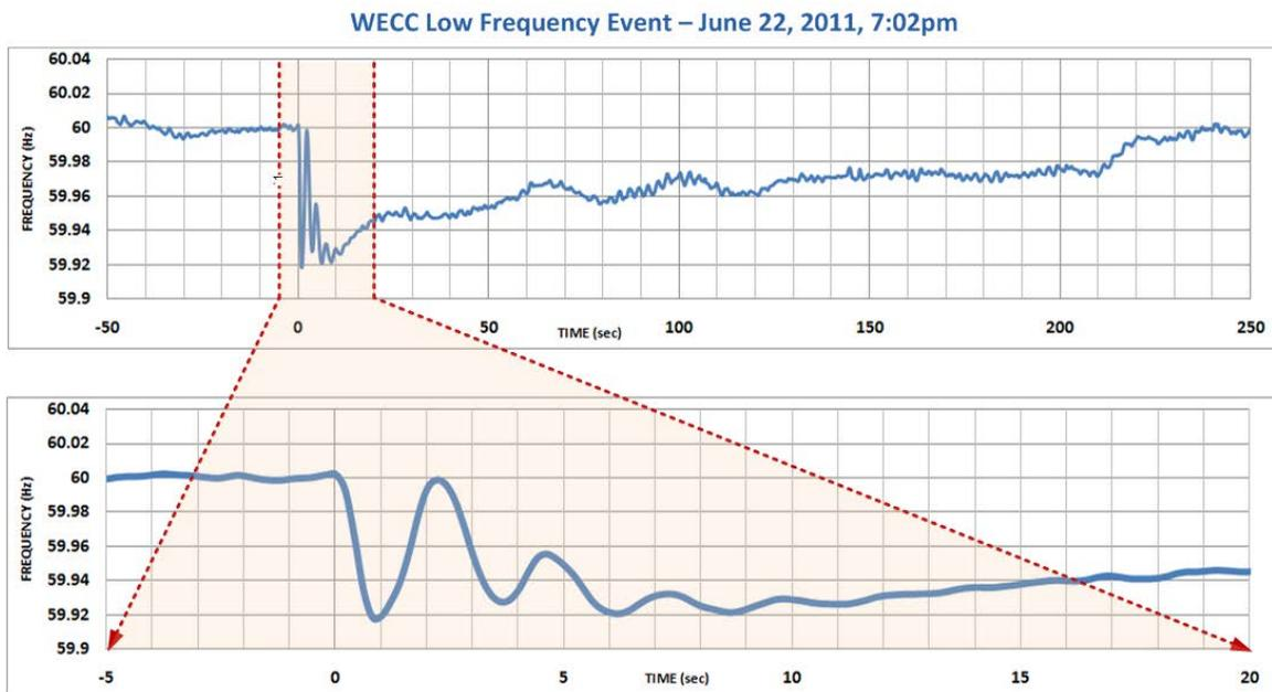
Figure 3-32. Example of WECC event with oscillations.
