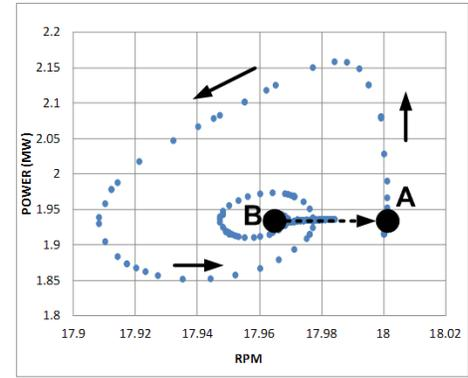
**Figure 3-9. Trajectory of operating point during a frequency decline for Type 1 WTG for a system with low inertia.**
