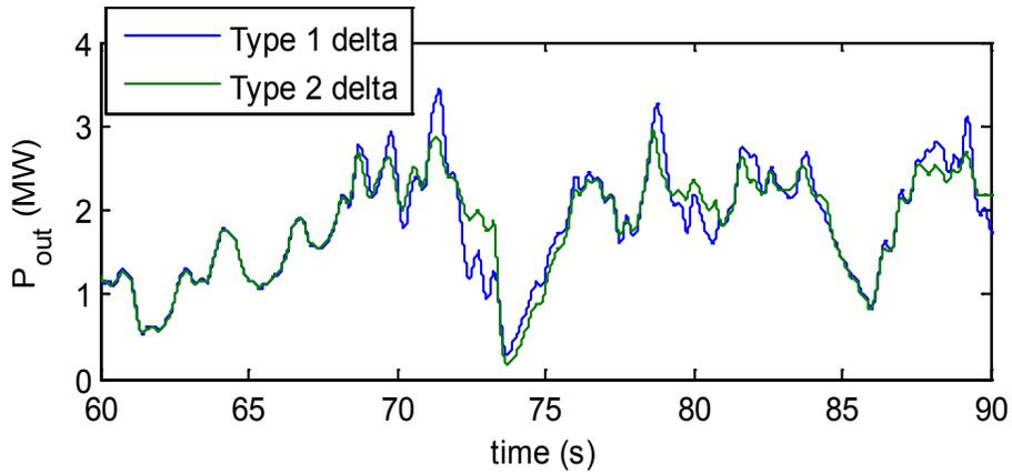
Figure 3-16. Output power comparison between the output power of a Type 1 wind turbine and that of a Type 2 wind turbine with  $\Delta P_{reserve} = 20\%$  of the rated power in time domain.
