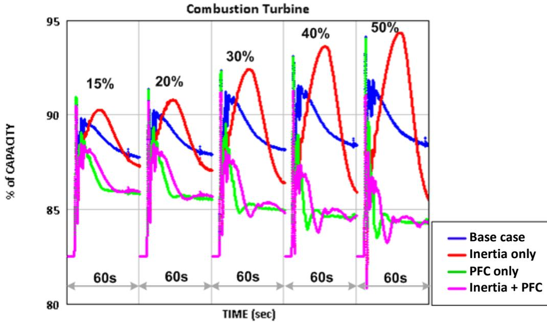
Figure 3-50. Frequency response contribution from combustion unit.
