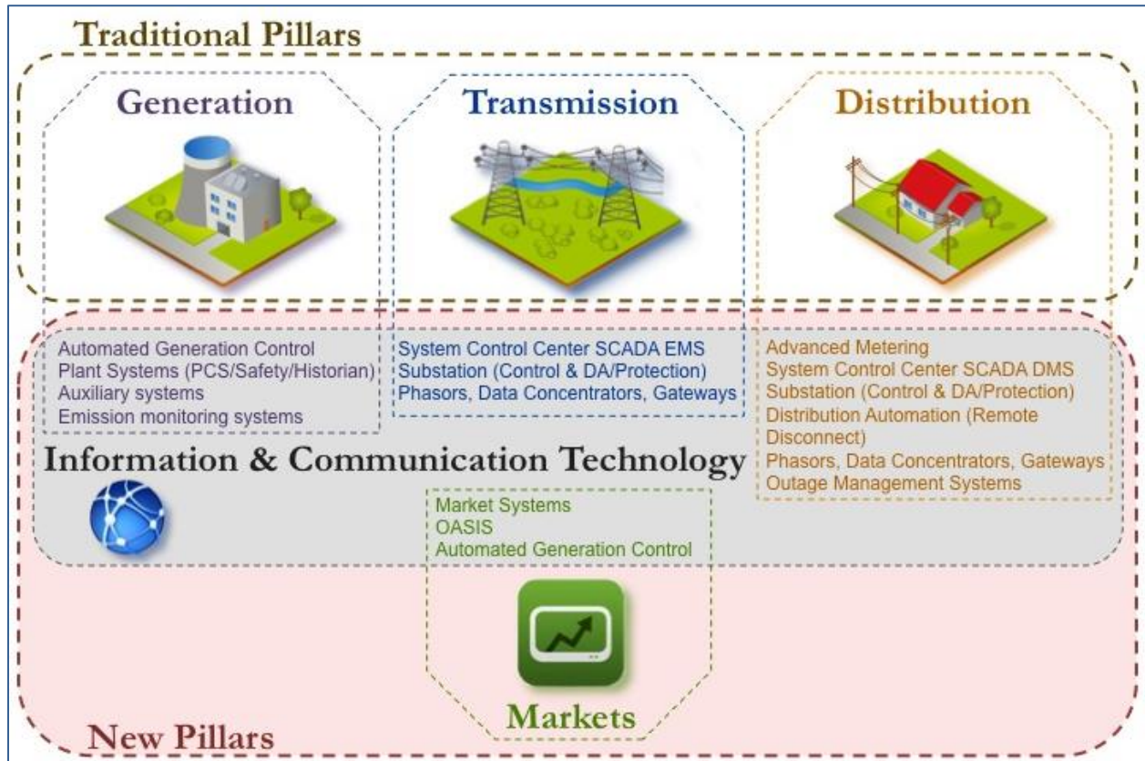
Figure 1.1. Five Pillars of the Electric Power Sector
