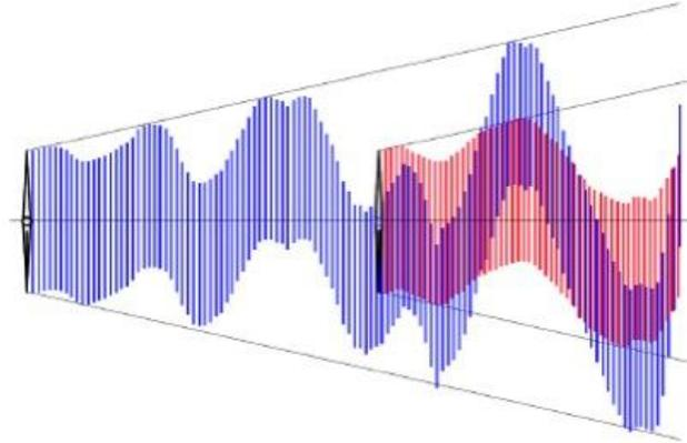
The wakes from two turbines (or more) only rarely coincide. Even in full wake direction, the path's will be different.
