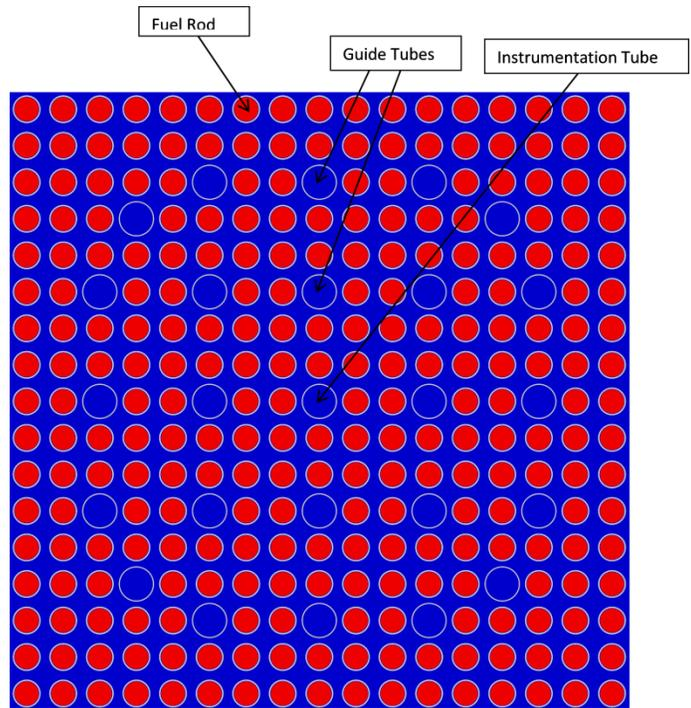
Figure 8-1. Cross-sectional model view of a Westinghouse 17 × 17 OFA and STD fuel assembly
