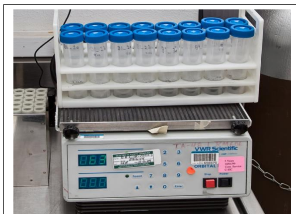
Figure 5-3. Granodiorite batch adsorption-desorption experiment setup.
