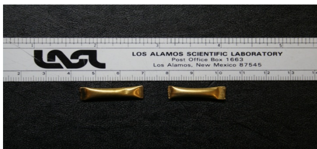
Figure 8. Examples of gold capsules prepared for high temperature, pressure (300 °C, 150 bar) experimental sulfate runs.
