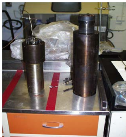
Figure 7. Bridgeman seal-type pressure vessel for 300°C, 150 bar hydrothermal experiment
