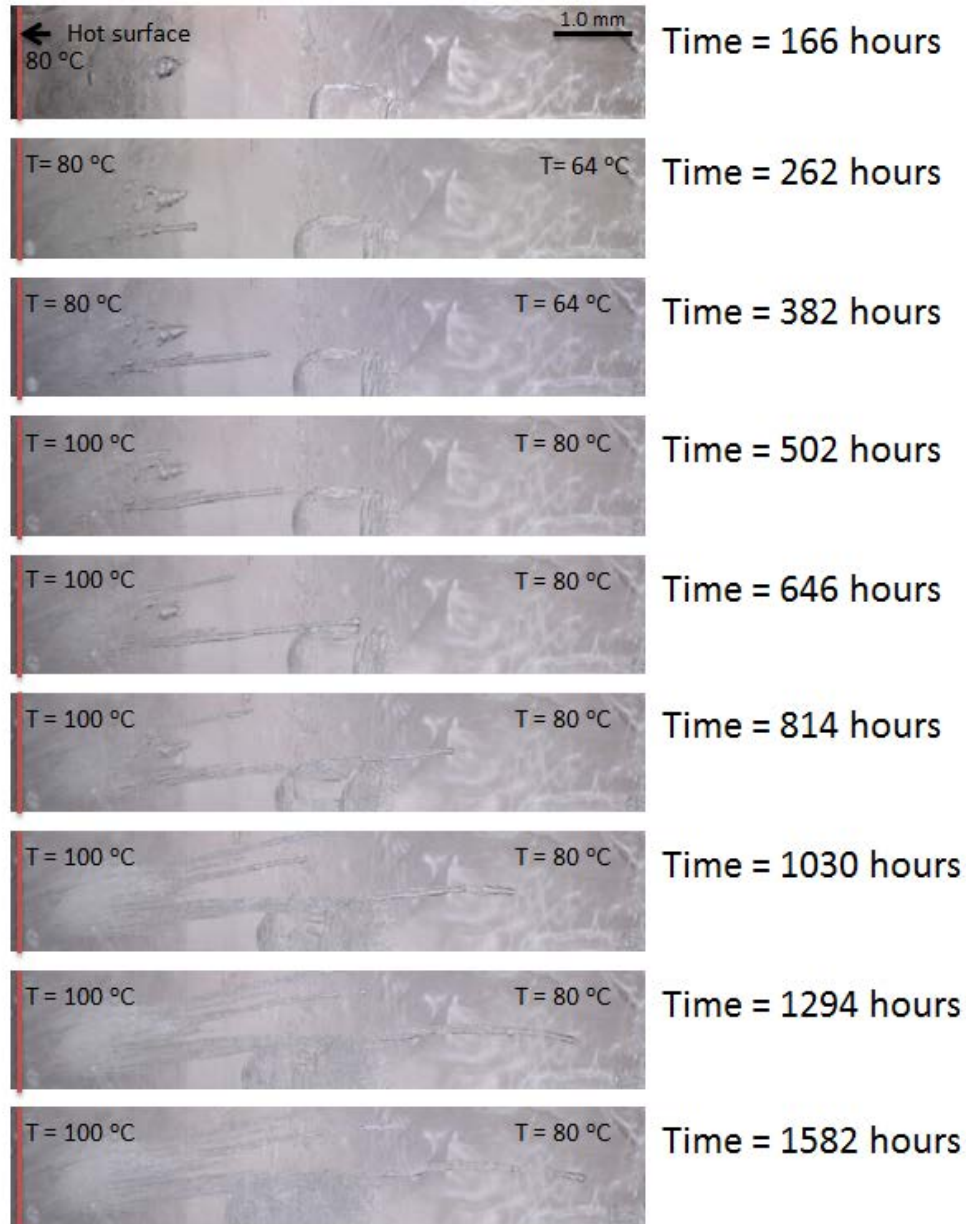
Figure 41. Images showing the migration of the gas phase to the cooler side of the salt crystal through narrow migration channels. Temperature at the hot end of the salt is 80 °C initially and then increased to 100 °C. Temperature at the cooler side is as indicated on the images.
