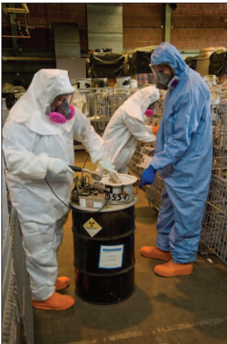
Radiological control technicians and material handlers check Alpha 5 containers before disposal
