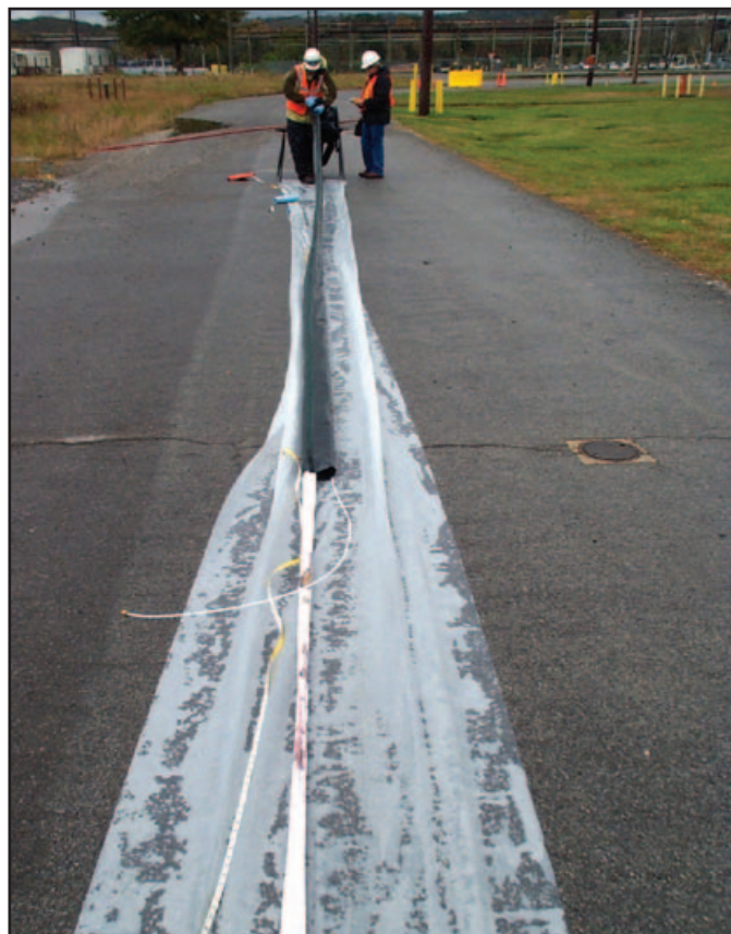
A liner impregnated with indicator chemicals was inserted in boreholes to determine the presence of DNAPLs. The purple stain indicates that DNAPLs contacted the liner.
