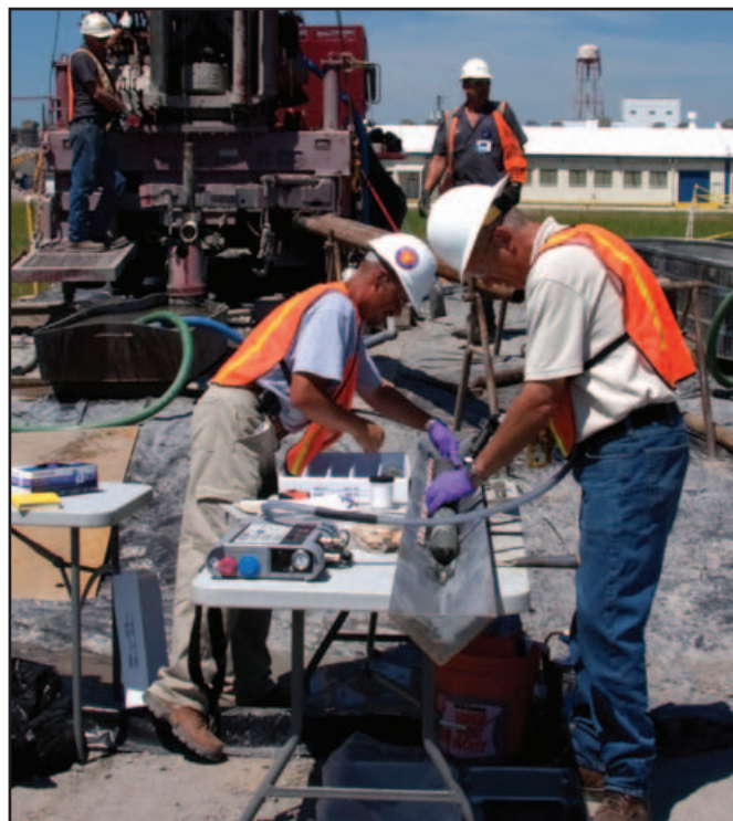
Workers scan drill corings to detect contaminants
