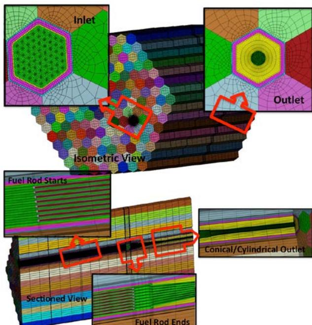
Fig. 6. EBR-II core model created with MeshKit. This version targets the XX09 test assembly for higher resolution.
