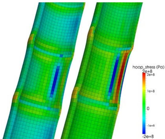
*Fig. 4. Modeling of hoop stress in pellet with surface defect: (left) no contact and (right) glued contact.*
