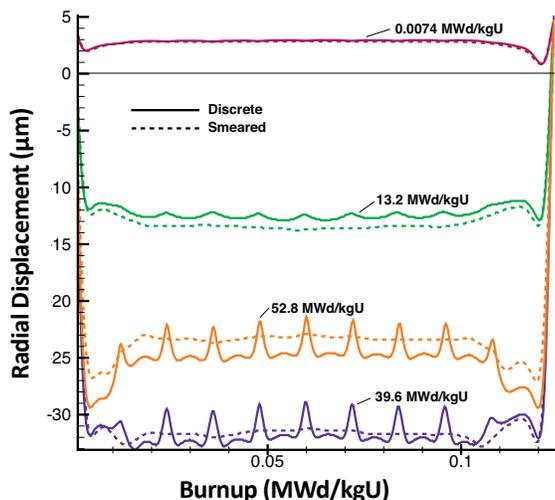
*Fig. 3. Cladding radial displacement versus axial length over time.*
