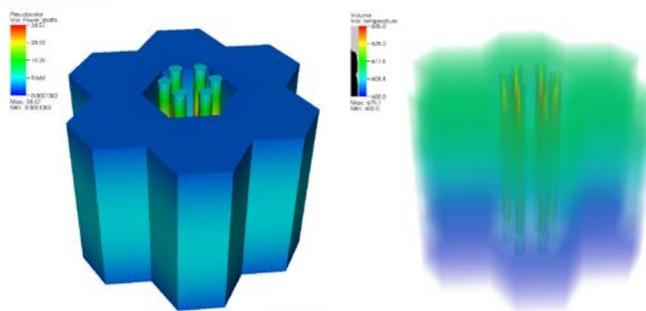
*Fig. 5. Simplified six-assembly multiphysics simulation of both power (left) and temperature (right).*
