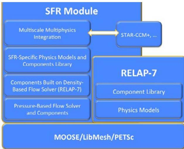
Fig. 7. Structure of the SFR systems analysis module.
