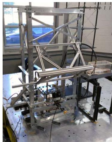
The photo on the left shows a seismic testing facility under construction at George Washington University. This unique facility can shake a full-scale fuel assembly and measure subsequent changes in its form and structure. It very accurately mimics the motion of the earth during a wide range of earthquake scenarios.
