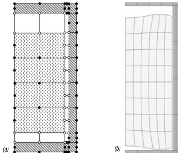
**Fig. 1.** (a) Axisymmetric legacy model of fuel and cladding with 8-node finite elements. Open circles are paired nodes connected with 1D elements. (b) Finite element model for which 1D node-to-node connections cannot be made.
