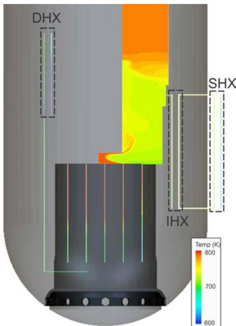
Fig. 8. Temperature distribution obtained in a coupled simulation of an SFR protected loss-of-flow transient.
