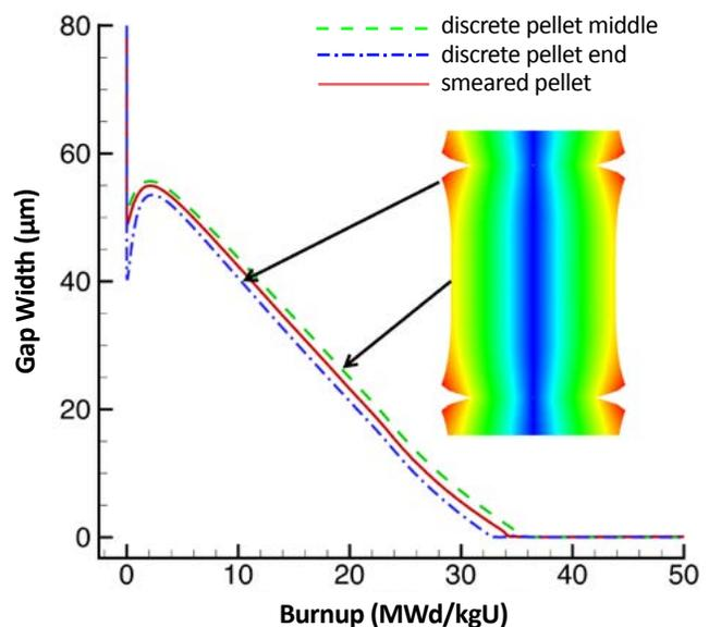
**Fig. 2.** Gap closure simulated by smeared and discrete pellet models. Inset coloring represents radial displacement.
