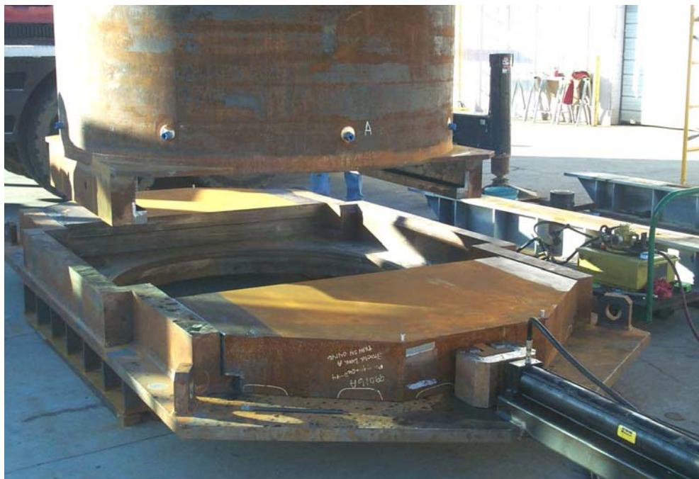
Figure 5-3 NAC Adaptor Plate Door Operation (NAC SNFDS Seminar)
