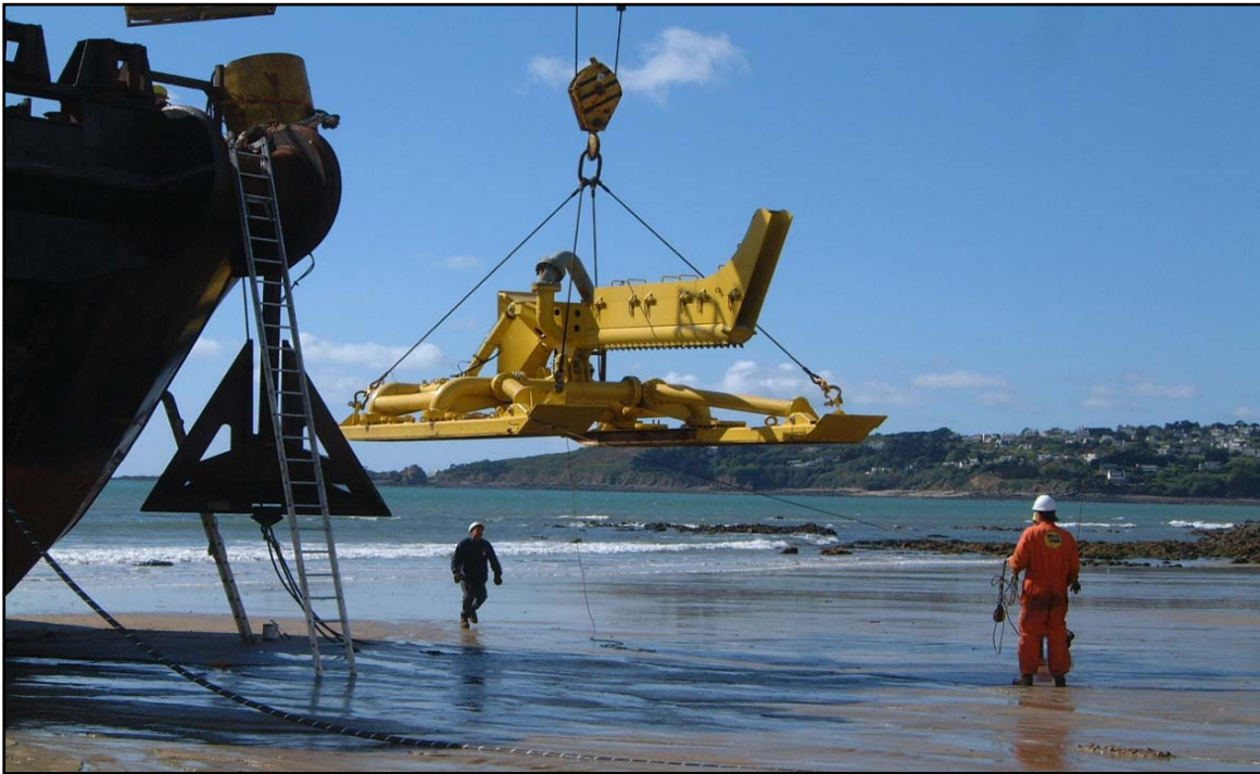
Figure 2-15. Example of Water Jet Trenching Device
