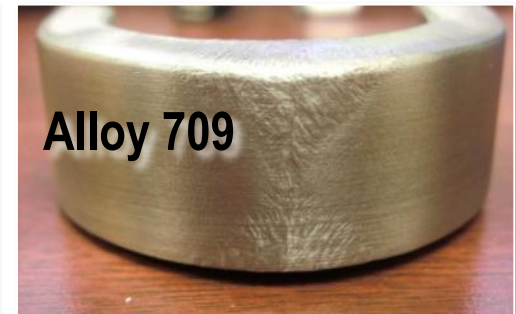
No visible defects in welds after 4t bend
