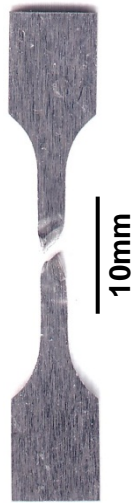
Sub-sized specimen (after testing at RT)
