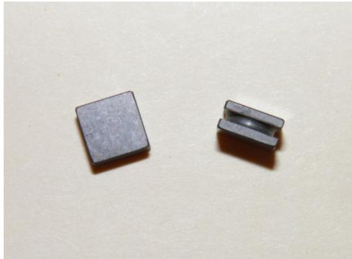
*Miniature torsion specimens of Ti diffusion-bonded SiC joints*
