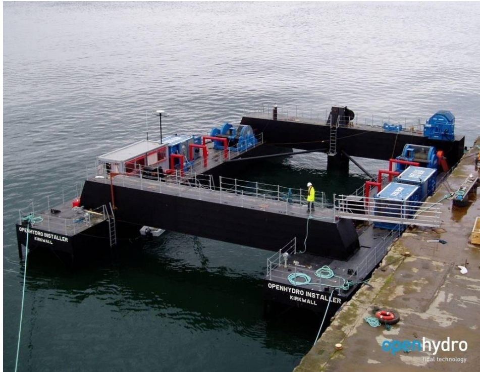
Figure 3. OpenHydro Installation Barge (Source: application).
