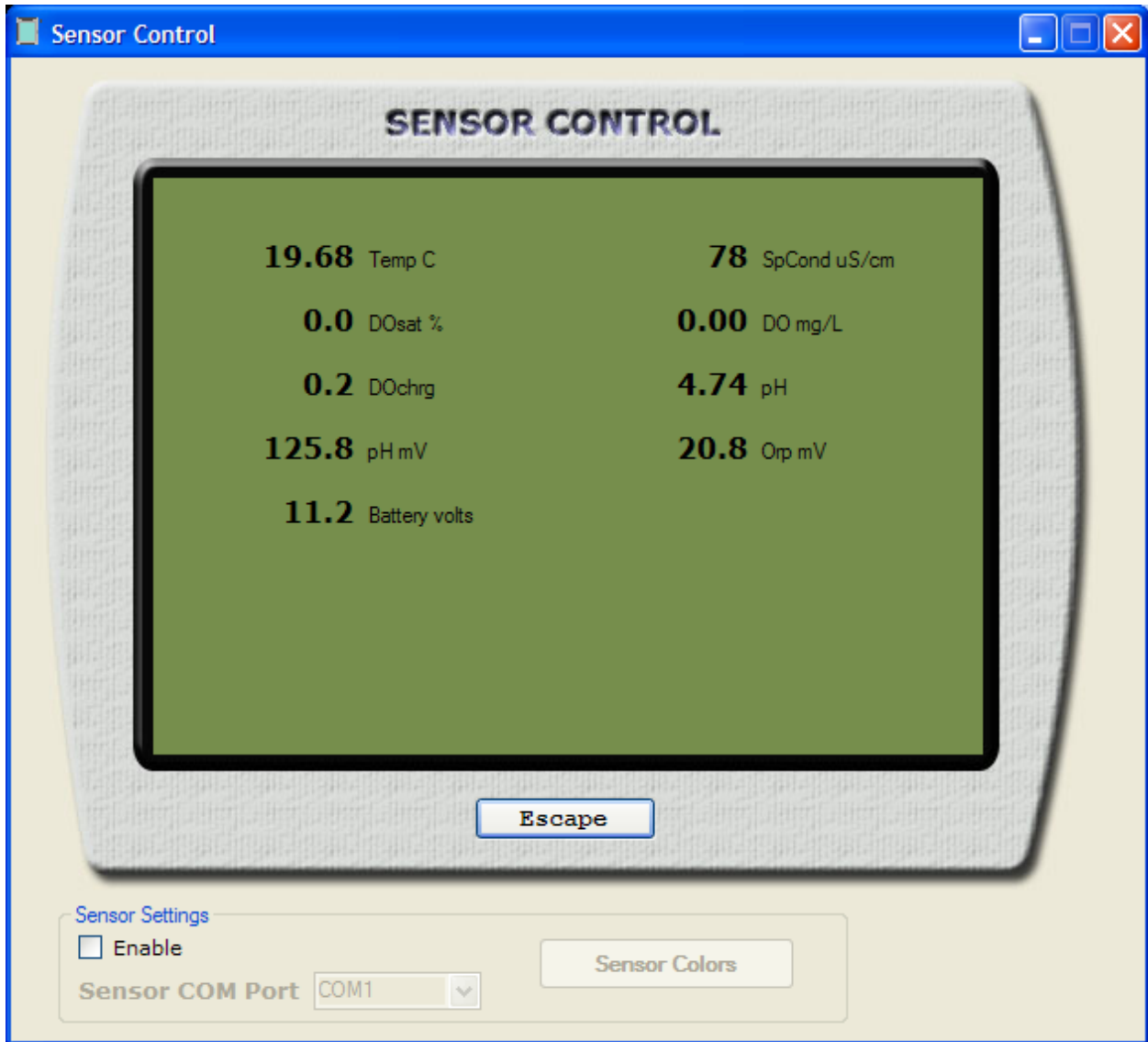
Figure 18. Sensor Control Window Displaying Live Readings
