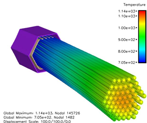
Fig. 2. Predicted deformations in the EBR-II XX09 assembly during an SHRT pseudo-transient simulation. Displacements are exaggerated 100-fold.
