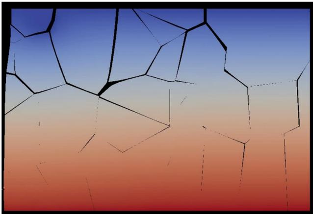
Fig. 1. Mesoscale simulation of fractures in  $UO_2$  fuel.
