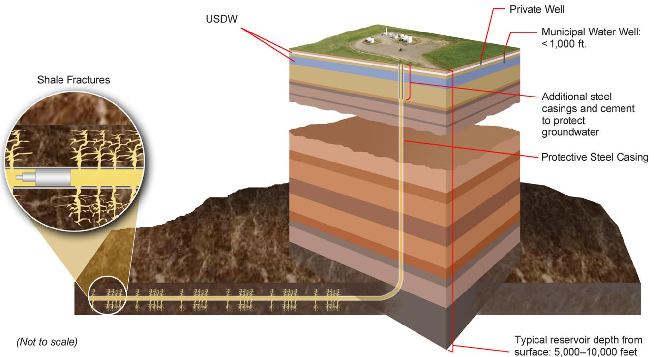
*Producible portions of shale gas formations are located many thousands of feet below the surface, well below groundwater aquifers. Modern hydraulic fracturing technology involves sophisticated engineering processes designed to create distinct fracture networks in specific rock strata. Experts continually monitor all aspects of the process, which must comply with local, state and federal laws and regulations.*
