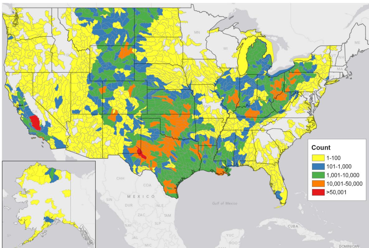
More than 4 million oil and gas related wells have been drilled in the United States since development of these energy resources began nearly 150 years ago. At least 2 million of these have been hydraulically fracture-treated, and up to 95 percent of new wells drilled today are hydraulically fractured, accounting for more than 43 percent of total U.S. oil production and 67 percent of natural gas production.
