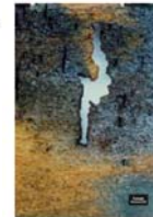
Washout caused by pitting and corrosion fatigue in a drill pipe
