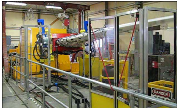
Figure 2-6. NREL Universal Resonant Excitation System
