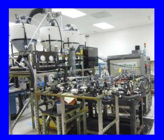
Flow Battery Prototype
