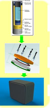
Traditional tubular Na – sulfur cell, operated >300-350°C
