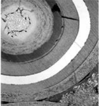
Particle with cracked IPyC layer
