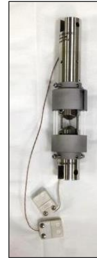
Double-contained specimen grips for elevated-temperature tensile tests.
