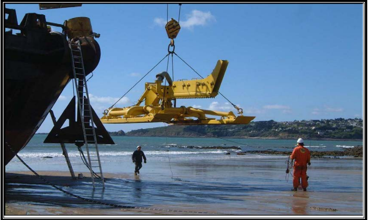
FIGURE 2-11 EXAMPLE OF WATER JET TRENCHING (JET PLOW) DEVICE
