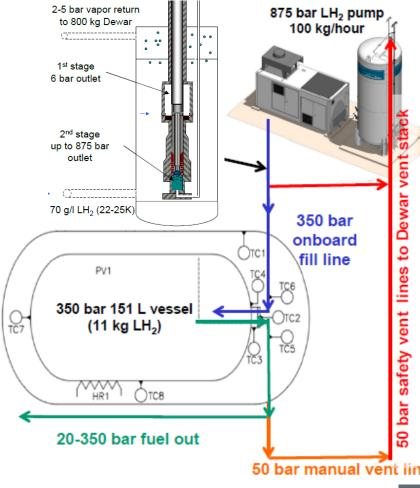
(above) Cryocompressed H<sub>2</sub> distribution concept.<sup>1</sup> (left) 5.6 kg Cryocompressed H2 tank cost estimate.<sup>2</sup> (center) 5.6 kg Cryocomp. tank volume distribution.<sup>2</sup>
