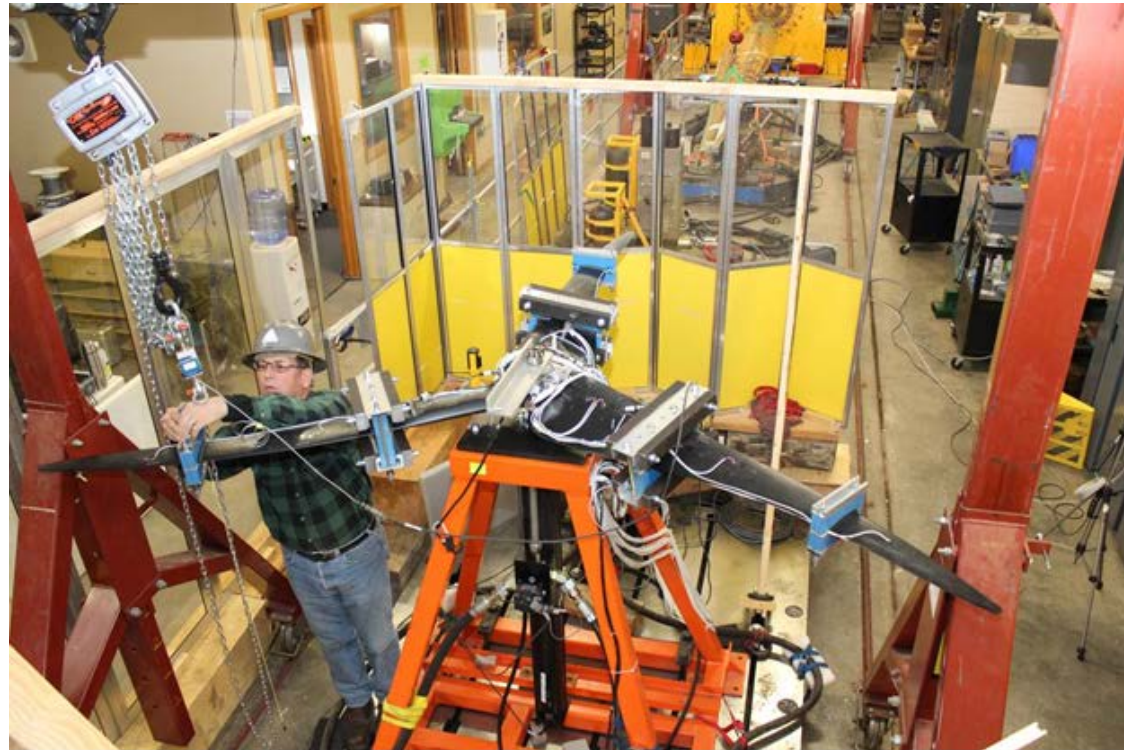
Rotor Fatigue Test for Pika at NWTTC
