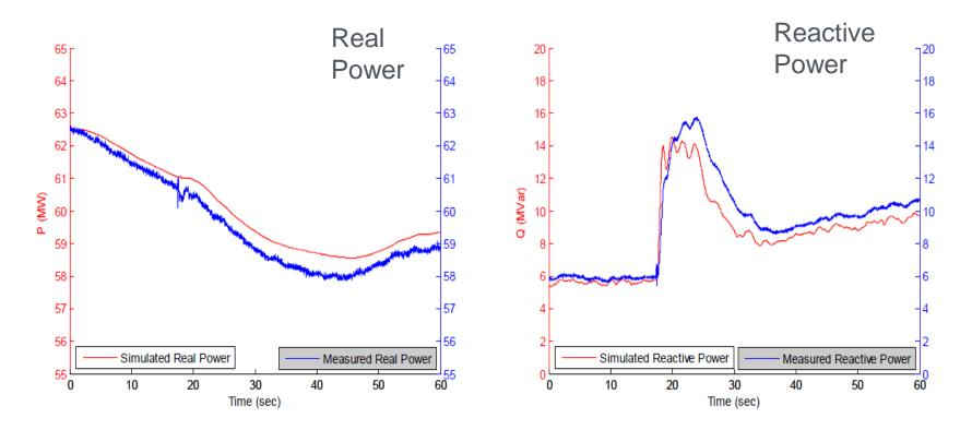
An example of dynamic model validation (measured data vs. simulated data)
