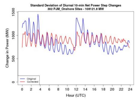
Figure 3. Diurnal mean standard deviation of 10-minute net power deltas from 302 onshore sites within the PJM region before (blue) and after (red) the diurnal correction was applied for the years 2004-2006.
