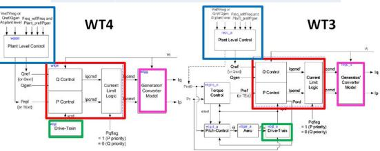
Block diagram of type 3 and type 4 WTG models
