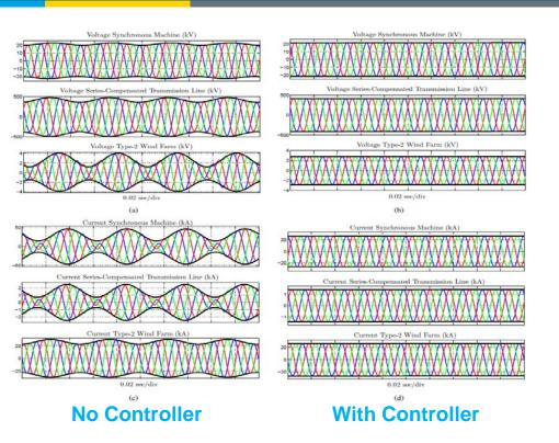
Subsynchronous Resonance at a Wind Power Plant (Recorded)
