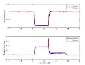
Modeled and measured comparison of a type 4 WTG response to a voltage dip at high side of step-up transformer.
