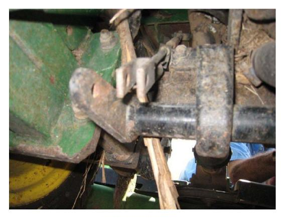
Figure 2-8: Disconnected Tie Rod (and Missing Pin) with Stick Wedged in Frame
