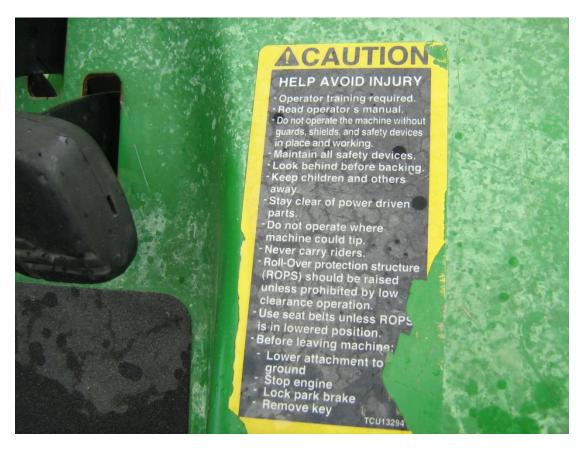
Figure 2-11: Warning Label found on the Front of Mower 1
