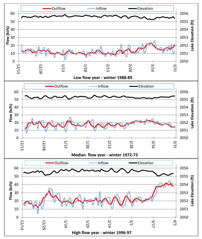
Figure 4-3. No Action Alternative Operations Inflow, Outflow, and Lake Elevation with MCE of 2055 feet for Low (10<sup>th</sup> percentile), Median (50<sup>th</sup> percentile), and High (90<sup>th</sup> percentile) Flow Years.
