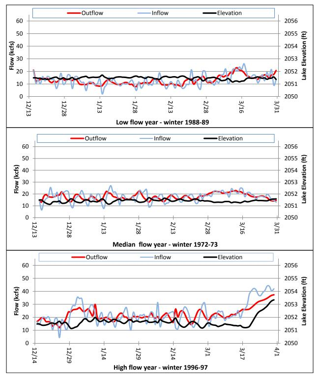
Figure 4-2. No Action Alternative Operations Inflow, Outflow, and Lake Elevation with MCE of 2051 feet for Low (10<sup>th</sup> percentile), Median (50<sup>th</sup> percentile), and High (90<sup>th</sup> percentile) Flow Years.
