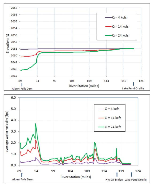
Figure 4-5. Modeled Stage and Velocity (non-ice conditions) in the Pend Oreille River between Lake Pend Oreille and Albeni Falls Dam when Lake Pend Oreille is 2051 feet as measured at Hope.
