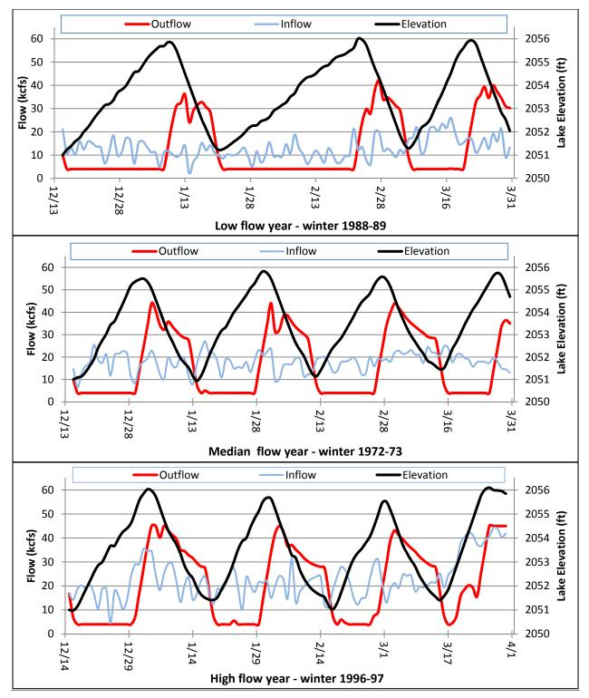
Figure 4-1. Flexible Winter Power Operations Inflow, Outflow, and Lake Elevation for Low (10<sup>th</sup> percentile), Median (50<sup>th</sup> percentile), and High (90<sup>th</sup> percentile) Inflow Years.
