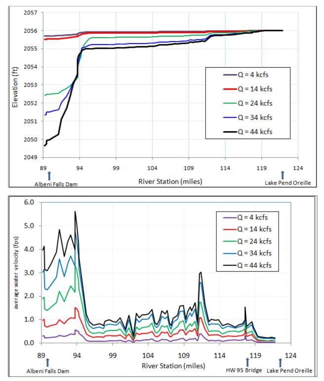
Figure 4-6. Modeled Stage and Velocity (non-ice conditions) in the Pend Oreille River between Lake Pend Oreille and Albeni Falls Dam when Lake Pend Oreille is 2056 feet as measured at Hope.
