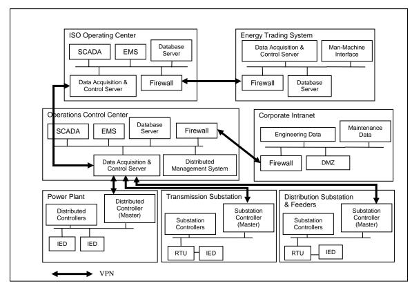
Figure 1: Levels of a Control System Architecture
