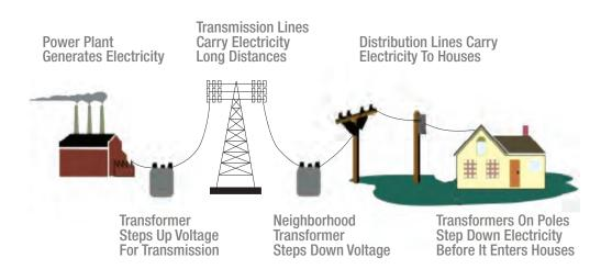
FIGURE 3: ELECTRICITY TRANSMISSION FROM GENERATION TO POINT OF USE 7
