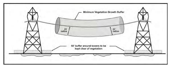
Figure 2-3. Buffered Vegetation Management Approach for 230-kV Line
