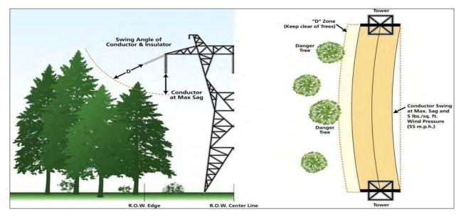
Figure 2-6. Conductor Swing
