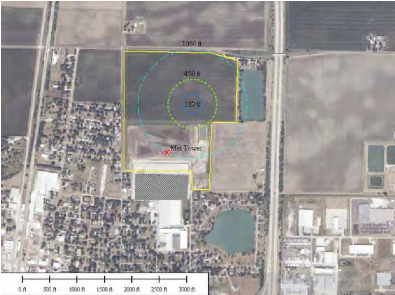
Figure 1- Libman turbine and setbacks
