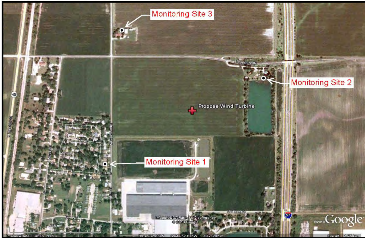
Figure 3-4. Monitoring Sites for Measuring Baseline Sound Conditions
