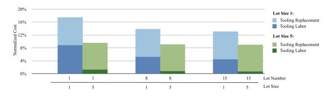
Figure 7: Normalized Cost Contributions By Tooling Labor and Tooling Replacement Cost Categories for Two Lot Sizes.
