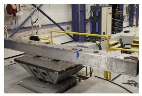
Figure 2. Basket-containing assembly with instrumented surrogate fuel rods placed upon a shaker to simulate vibrational and shock loading associated with a normal 700-mile truck journey.
