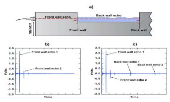
Figure 2. a) Illustration of ultrasonic energy propagating through a stainless steel baseplate and reflecting off of drain sump surfaces (i.e., front wall and back wall). Depiction of signals containing b) features of multiple front wall echo signals for the condition of an empty drain sump and c) features of multiple front wall and back wall echo signals for a drain sump containing water.
