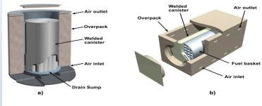
Figure 1. Illustrations of generalized dry storage systems consisting of a welded stainless steel canister and concrete overpack. Two types of systems are distinguished by orientation of the canister a) vertically and b) horizontally.
