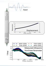
Figure 2. Example of nonlinear ultrasonic parameter measured as a function of time as specimen was subjected to hightemperature creep. The graphic also shows the arrangement of the transducers for applying the excitation and recording the response.
