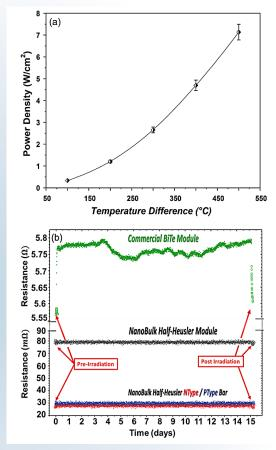
Figure 3. (a) Electric power density versus temperature difference of a nanobulk half-Heusler unicouple device at a constant cold-side temperature of 100°C. (b) Gamma radiation effect on the electric resistances of the nanobulk half-Heusler devices and a commercial BiTe device.
