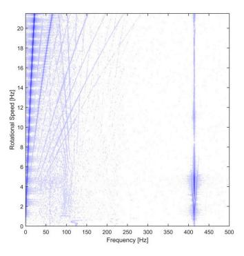
Figure 6. Waterfall plot of rotordynamics
