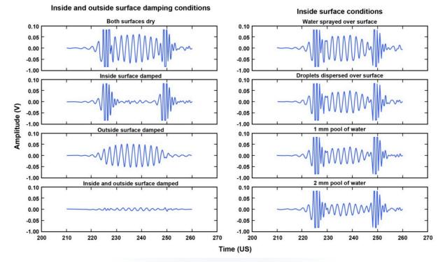
Figure 5. Receiver responses – left series: progressive waveforms for both sides dry, inside (top) surface damped, outside (bottom) surface damped, and both surfaces damped; right series: both sides dry, inside (top) surface droplets, 1 mm, and 2 mm of water on plate top surface.
