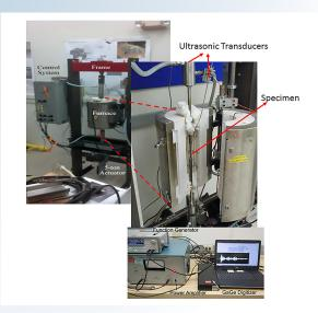
Figure 1. Accelerated aging test-bed with in-situ online condition monitoring sensors.
