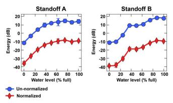
Figure 3. The back wall echo signal energy as a function of the water level in the sump at two different standoffs near the top of the drain sump. Results for back wall echo signal normalized to front wall echo signal are provided (red) along with the signal with no normalization (blue).
