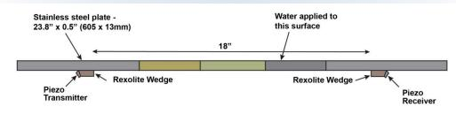
Figure 4. Illustration of experimental set-up used to demonstrate capability to detect small quantities of water on the surface of stainless steel plate opposite to the surface that transducers are mounted.
