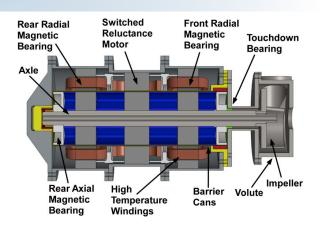
Figure 2. Concept drawing of a canned-rotor, magnetically suspended, reluctance drive motor-pump.
