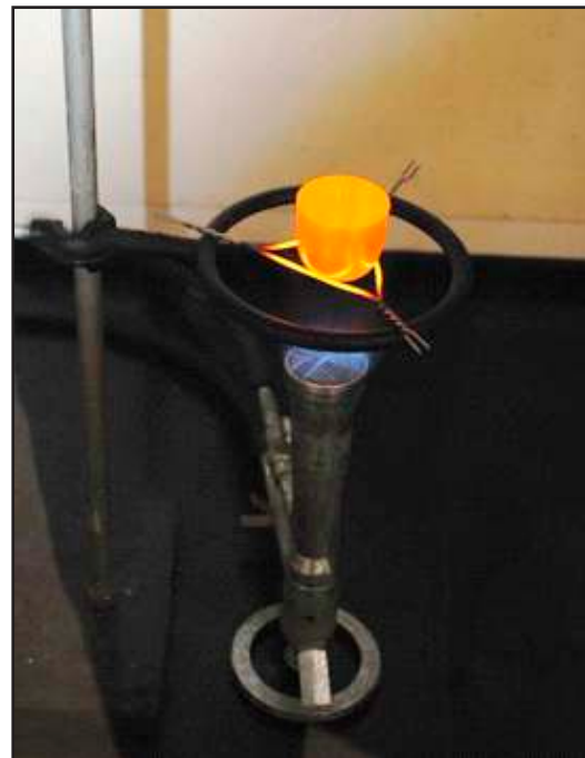
A soil sample is dissolved in a flux at high temperature.
