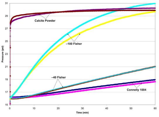
Figure 3. Reproducibility of Reactivity Tests Using Standard ZVI Samples
