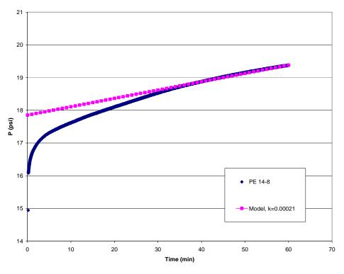
Figure 9. Typical Reactivity Test With Model Curve Fitted to Match Slope at 60 Minutes (The rate constant in this example is 0.00021/per min. The unitless reactivity value is 2.1. The sample clearly has some carbonate as indicated by the rapid, early increase in pressure.)
