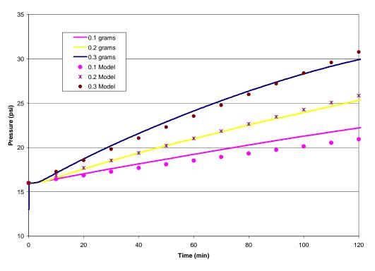
Figure 7. Model Fit to Three Different Masses of Fisher -40 Mesh ZVI
