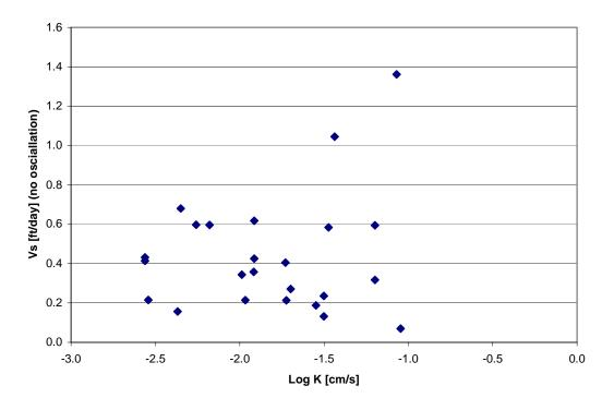
Figure 17. Well Screen Velocity Versus Hydraulic Conductivity Relationship
