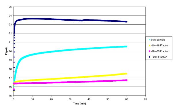
Figure 10. Reactivity Curves for Bulk Sample PE-ZVI-3-4 and Various Size Fractions
