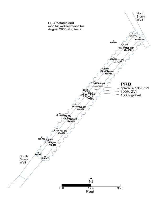
Figure 11. Locations of August 2003 Slug Tests at Monticello PRB
