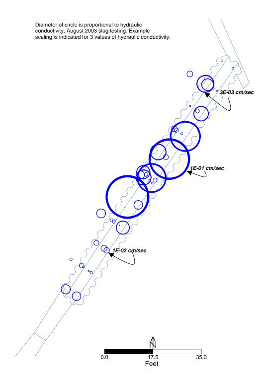
Figure 13. Graphical Representation of Hydraulic Conductivities Determined From August 2003 Slug Tests at Monticello PRB (circle size proportional to hydraulic conductivity)
