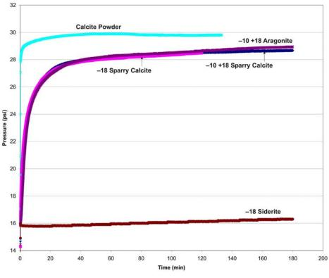
Figure 5. Reactivity Curves for Carbonate Minerals
