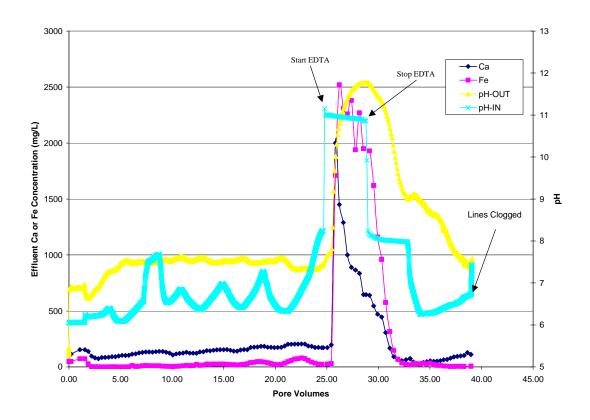
Figure 20. Results of Rejuvenation Column Test Using EDTA
