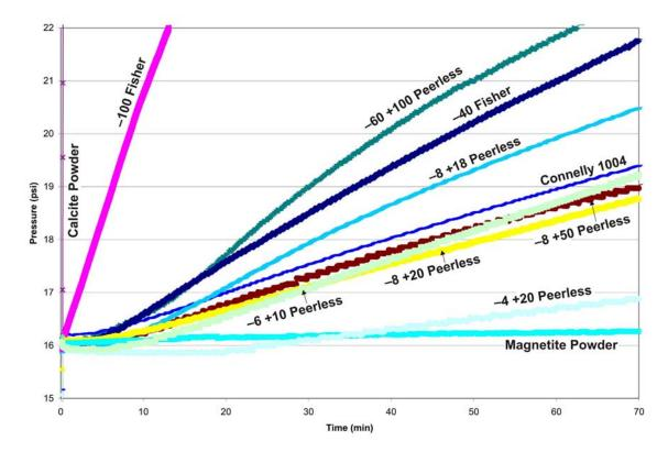
Figure 4. Reactivity Curves for a Variety of ZVI Types
