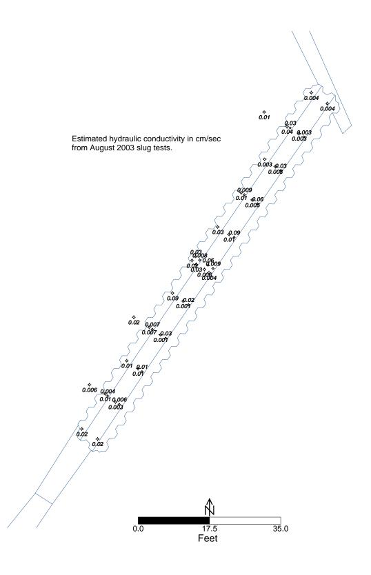
Figure 12. Estimated Hydraulic Conductivity (cm/s) Calculated From August 2003 Slug Tests at Monticello PRB
