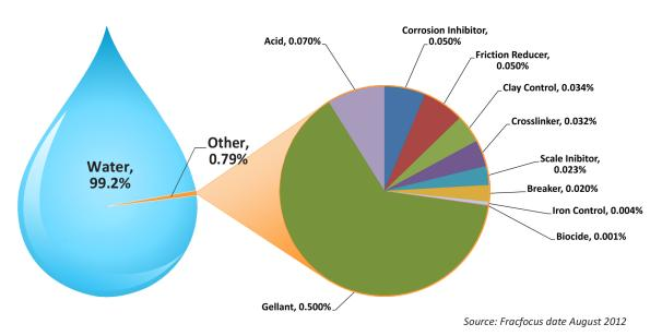
Slickwater is mostly water, with a relatively consistent 0.5 to 2.0 percent comprised of additives.
