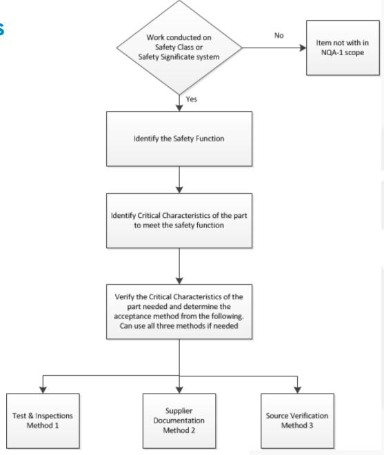
Overview: CGD consists primarily of an Engineering evaluation to establish critical characteristics for acceptance based on the safety function(s) of an item. Dedication is performed on items obtained from a Supplier who does not have a Nuclear QA Program.
